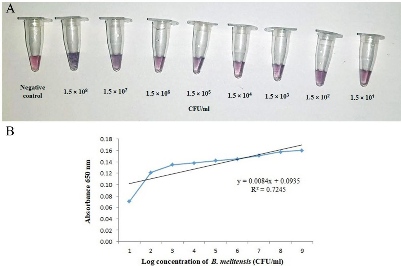
**Fig. 5** (A) Aptasensor sensitivity for the detection of *Brucella* cells from  $1.5 \times 10^1$  to  $1.5 \times 10^8$  CFU/mL. (B) Linear dependence between the OD values versus log *Brucella* cell numbers
