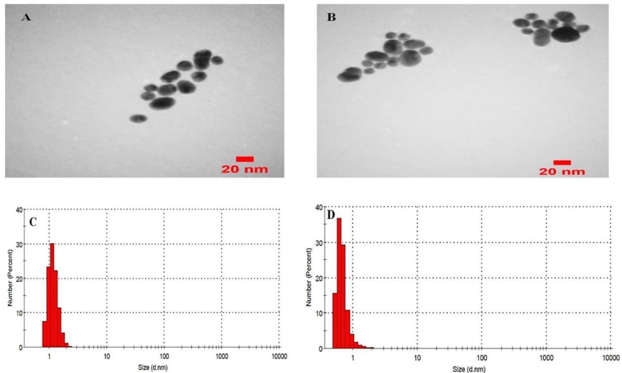
**Fig. 3** TEM micrograph: (A) synthesized GNPs. (B) GNPs coated with aptamer. DLS: (C) GNPs. (D) GNPs-aptamer
