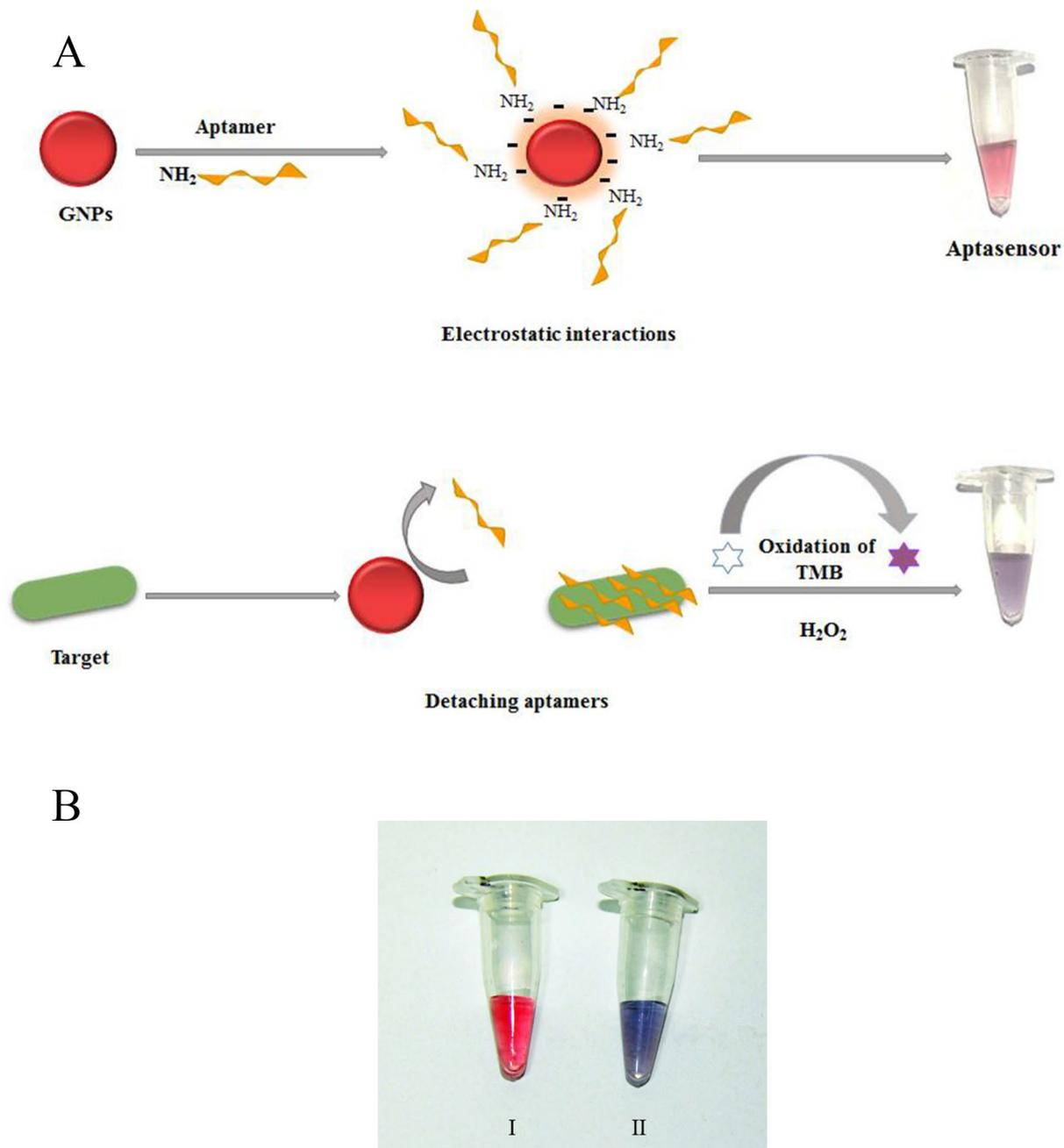
**Fig. 4** (A) Schematic illustration of the colorimetric reaction of the aptasensor to detect *Brucella* cell. (B) I: Reaction color in the absence of the bacterial cells. II: Reaction color in the present of the bacterial cells
