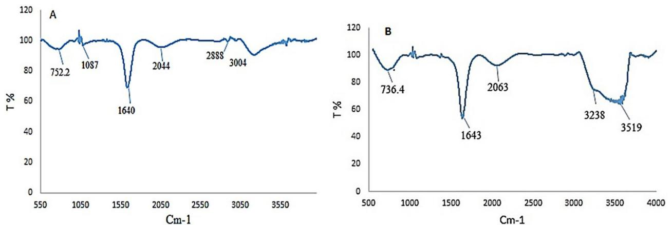
**Fig. 2** (A) FT-IR spectra of GNPs. (B) GNPs-aptamers
